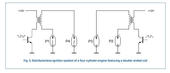
For some double-ended ignition coils, the driver transistor, which is responsible for controlling the primary winding current, would be located inside the coil housing, although it was usually located on the microprocessor board of the motor control unit. This transistor heats up excessively during operation, so changing its location was a favorable solution.
