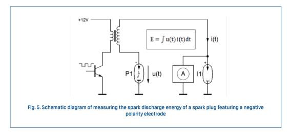
The method of measuring the spark discharge energy, the apparatus and the results of the exemplary testing are described in detail in publication [6]. Thanks to the uniform electrode polarization system shown in Figure 4, similar simultaneous measurement can be carried out for spark discharge on the remaining spark plugs.
